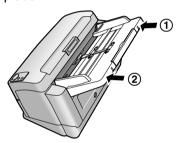
**c.** Pull out the feed extension tray in the direction of the arrow shown in the illustration below.
