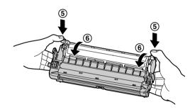
5 Make sure that the arrows (⑦) match, to install the toner cartridge correctly.
