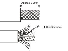
② Peel off the metallic shielded net and foil, and you will find 2 power cables (in red and black), 2 signal cables (in blue and white) and 1 shielded cable.
