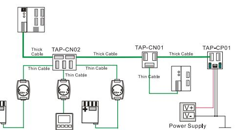
① To install TAP-CP01 at the starting point or end point of the network, you have to switch ON the termination resistance. To install TAP-CP01 in the middle of the network, you have to switch OFF the termination resistance.
