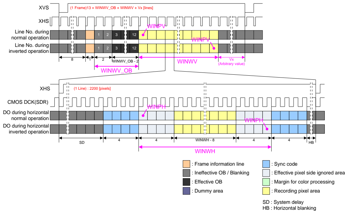
Drive Timing Chart for Window Cropping mode (Parallel CMOS output)
