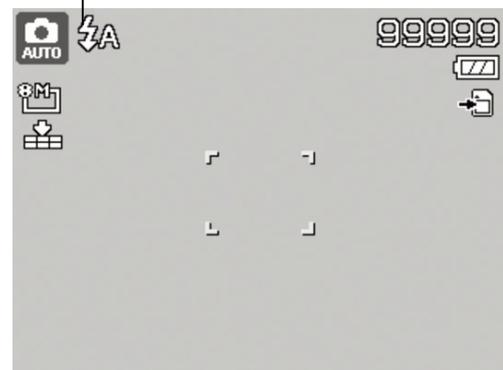
flash mode forces the camera to use a slower shutter speed in combination with the flash. The flash fires briefly to light the foreground (subject) while capturing ambient light to reveal more detail in the background. If Slow Sync flash is not used, the background may appear black or underexposed.
