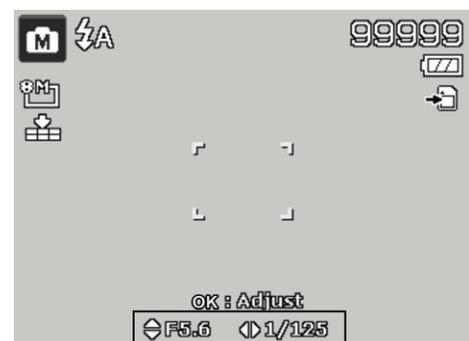
Displays the aperture and shutter speed value
