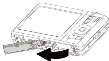
3. Insert the battery into the compartment with correct orientation as illustrated.
