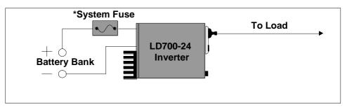
\* A system fuse (of at least 35 Amps) should be placed before the battery. An HRC motor start type is recommended. (See your system designer for details).
