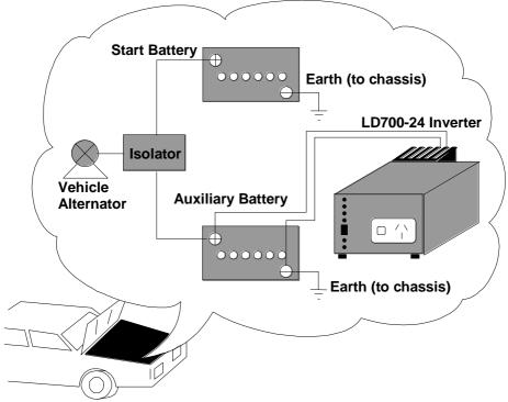
By incorporating an auxiliary battery in the manner above, the starting battery should remain charged for vehicle starting (see your auto electrician).
