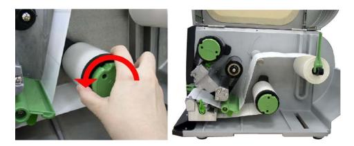
12. Lift up the peel-off roller release lever and close the print head mechanism.13. Move the peel-off sensor toward the paper exit chute.
