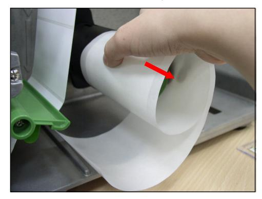
3. Then, slide off the liner from internal rewind spindle.
