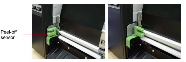
14. Peeling will automatically start. Press the FEED button to test.
