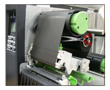
2. Push the ribbon release button to release the ribbon on the ribbon rewind spindle.
