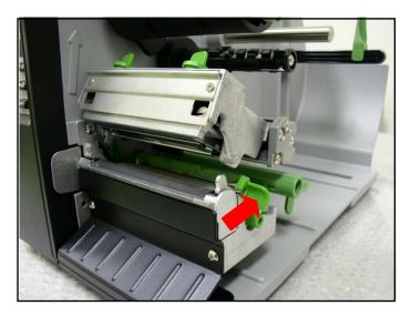
2. Move the label roll guard horizontally to the end of label spindle then flip down the label roll guard.
