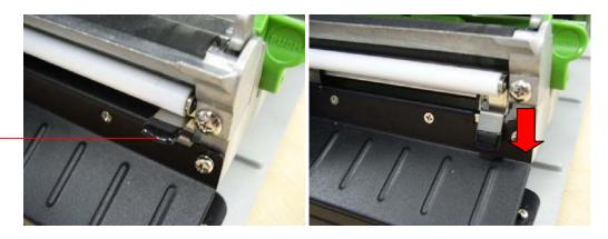
Peel-off roller release lever
