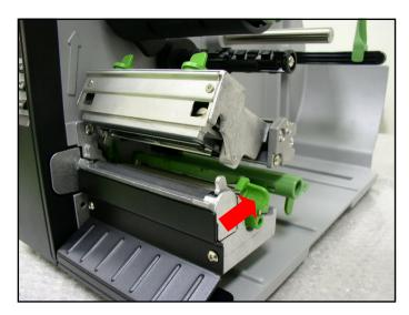
3. Install the ribbon onto the ribbon supply spindle.
