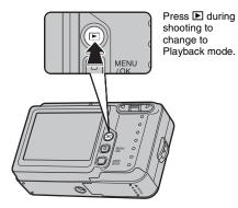
When the camera is off, press **D** for about 1 second to turn the camera on in Playback mode.
