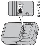
Press for about 1 second to turn the camera on in Playback mode.
