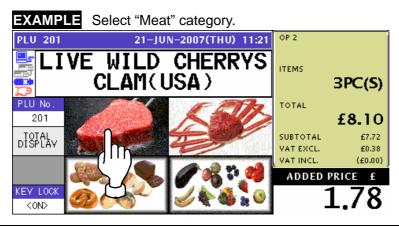
**5-2** The PLU preset screen for the selected category appears. Then, enter a desired PLU number using the numeric keys and press the [PLU] key on the key sheet, or simply press a preset key on the screen where a desired product is allocated.
