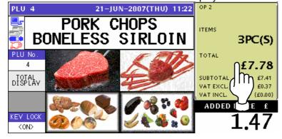
**7.** The detailed subtotal screen appears for confirmation of product registrations. Then, confirm that the detail of the transaction is correct
