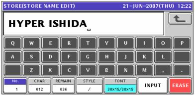
6. Press the [ESC] key on the key sheet to escape from text editing mode.
