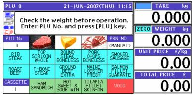
**2.** Enter a desired PLU number using the numeric keys and press the [PLU] key on the key sheet, or simply press a preset key on the screen where the product is allocated.
