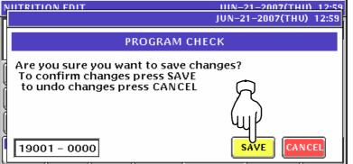
**9.** The edited text has been registered. When necessary, enter a nutrition data for each field using the numeric keys and press the corresponding field for registration.
