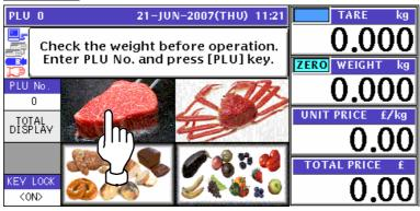
**5-2** The PLU preset screen for the selected category appears. Then, enter a desired PLU number using the numeric keys and press the [PLU] key on the key sheet, or simply press a preset key on the screen where a desired product is allocated.
