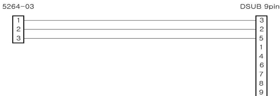
[Figure 5.11 COM2 Cable connection]
