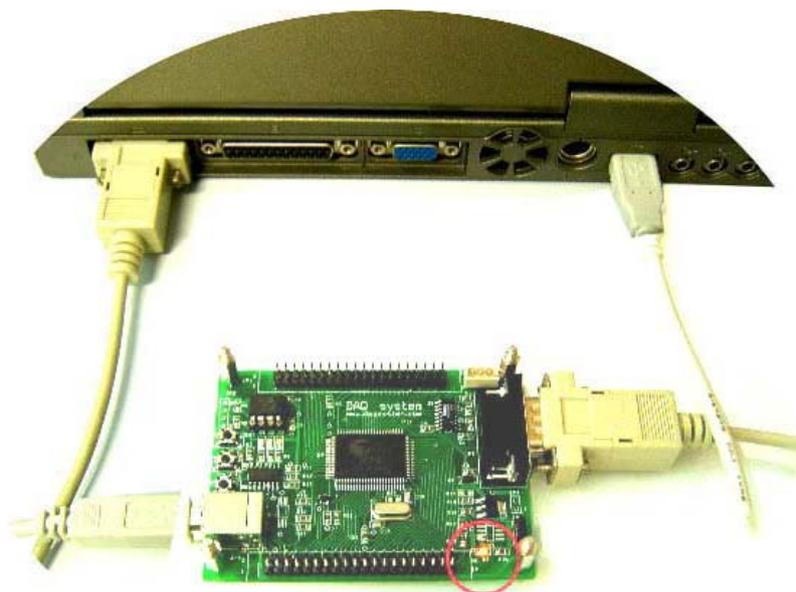
[Figure 5.2 USB-EK01 and PC connection using cable]
