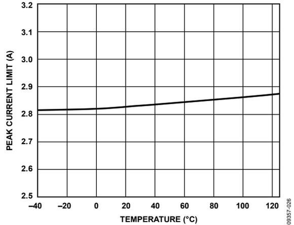
Figure 26. Current-Limit Threshold vs. Temperature,  $R_{ILIM} = 47 \text{ k}\Omega$
