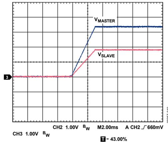
Figure 40. Ratiometric Tracking
