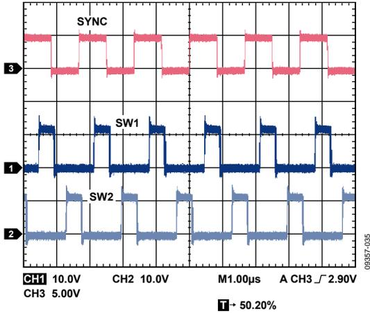
Figure 35. External Synchronization with 60° Phase Shift
