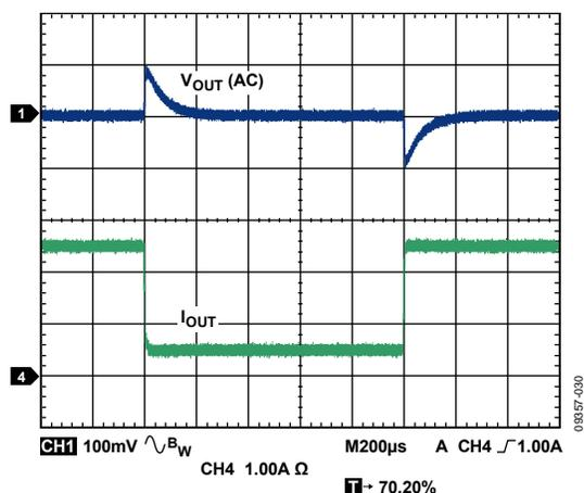
Figure 30. Load Transient Response, 0.5 A to 2.5 A
