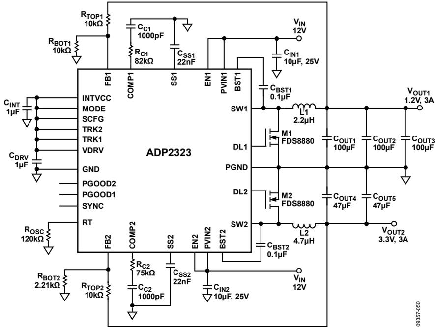
Figure 50. Using External MOSFET Application,  $V_{IN1} = V_{IN2} = 12\text{ V}$ ,  $V_{OUT1} = 1.2\text{ V}$ ,  $I_{OUT1} = 3\text{ A}$ ,  $V_{OUT2} = 3.3\text{ V}$ ,  $I_{OUT2} = 3\text{ A}$ ,  $f_{SW} = 500\text{ kHz}$
