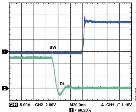
Figure 22. Low-Side Driver Falling Edge Waveform, C<sub>DL</sub> = 2.2 nF
