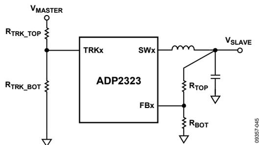
Figure 43. Voltage Tracking
