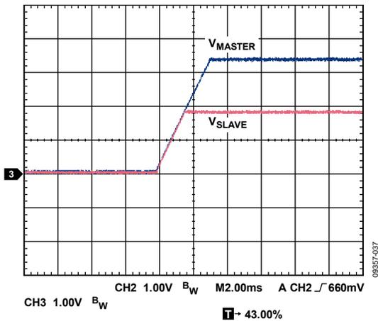
Figure 37. Coincident Tracking
