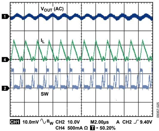
Figure 25. Discontinuous Conduction Mode (DCM)
