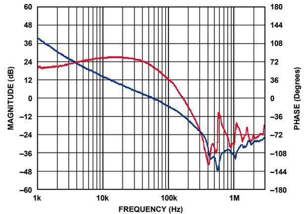
Figure 49. Bode Plot for 3.3 V Rail
