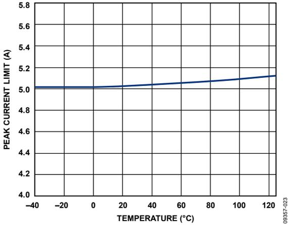
Figure 23. Current-Limit Threshold vs. Temperature,  $R_{ILIM} = \text{Floating}$
