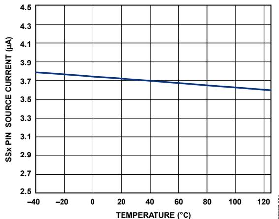
Figure 21. SSx Pin Source Current vs. Temperature
