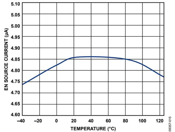
Figure 15. EN Source Current at  $V_{EN} = 1 V$
