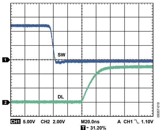
Figure 19. Low-Side Driver Rising Edge Waveform, C<sub>DL</sub> = 2.2 nF
