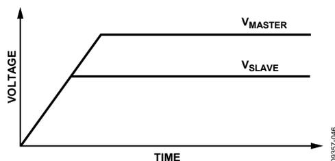
Figure 44. Coincident Tracking
