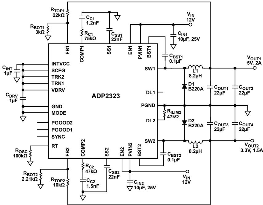
Figure 51. Using External Diode Application,  $V_{IN1} = V_{IN2} = 12\text{ V}$ ,  $V_{OUT1} = 5\text{ V}$ ,  $I_{OUT1} = 2\text{ A}$ ,  $V_{OUT2} = 3.3\text{ V}$ ,  $I_{OUT2} = 1.5\text{ A}$ ,  $f_{SW} = 600\text{ kHz}$
