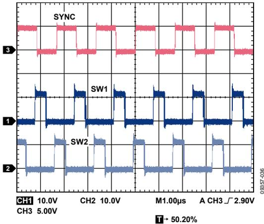
Figure 36. External Synchronization with 120° Phase Shift
