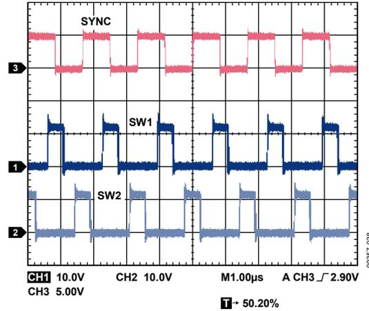
Figure 38. External Synchronization with 90° Phase Shift
