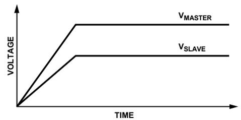
Figure 45. Ratiometric Tracking
