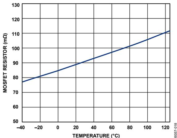
Figure 18. MOSFET R<sub>DS(on)</sub> vs. Temperature
