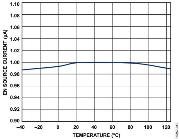
Figure 12. EN Source Current at  $V_{EN} = 1.5 V$
