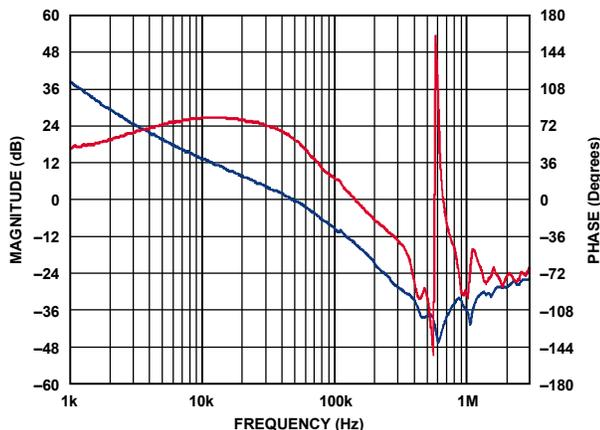
Figure 48. Bode Plot for 1.2 V Rail
