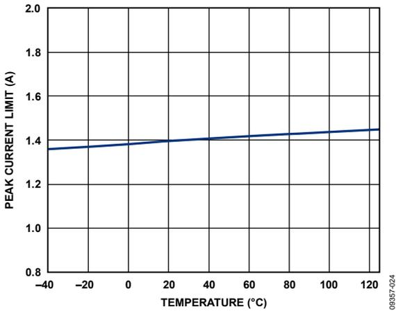
Figure 24. Current-Limit Threshold vs. Temperature,  $R_{ILIM} = 15 \text{ k}\Omega$
