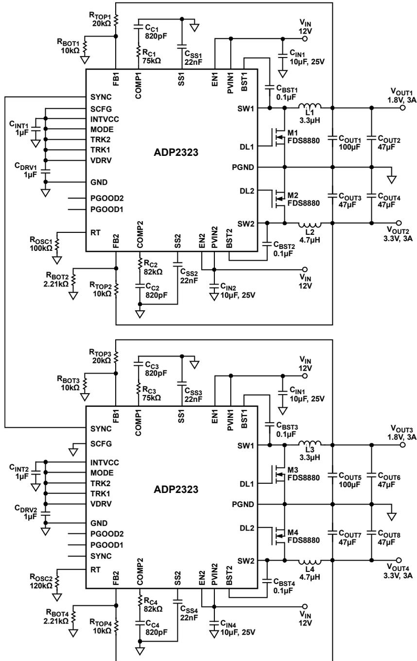
Figure 54. Synchronization with 90° Phase Shift Between Each Channel
