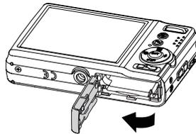
3. Insert the battery into the compartment with the terminal facing inside the camera.
