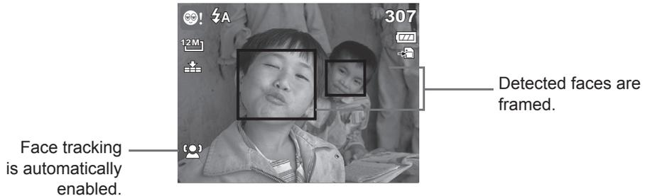
2. Press the shutter button half-way down to focus the subject. The frame turns green to indicate focus is set.
