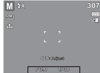
Displays the aperture and shutter speed value
