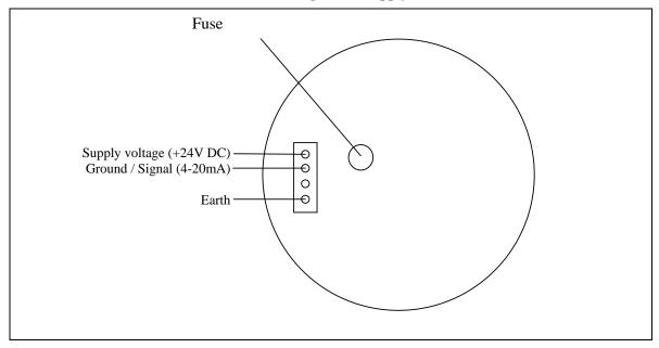
You can connect the EC35 directly to an evaluation unit by means of a 2-pole lead. The current consumption of the unit is approx. 25mA at an operating voltage of 24V DC.
