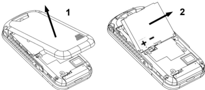
1. Insert your fingernail into the back cover slot on the bottom of the phone and lift off the back cover (1).
