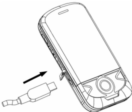
1. Connect the USB data cable into the cableless wall adapter.
