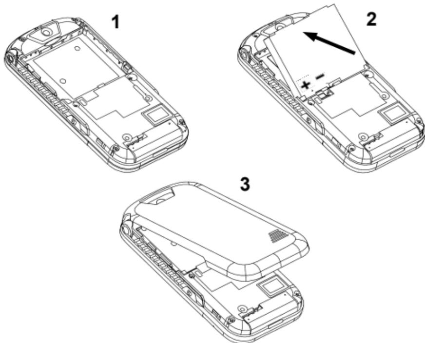
1. Insert the battery by aligning the contacts (1) and then gently press it down until it clicks into place (2).
