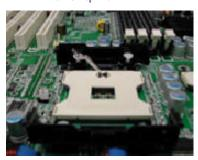
1. Pull the lever out, than lift up the Lever.
