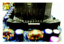
8. Hook one end of the cooler bracket to the CPU socket first.
