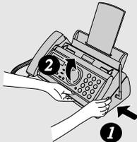
**2** Remove the used film and empty spool.
