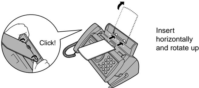
**Note:** The paper tray extension has a top side and a bottom side. If the tabs do not go into the holes, turn the support over.
