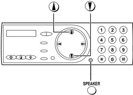
You can adjust the volume of the speaker, handset, and ringer using the up and down arrow keys.
