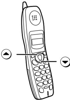
You can adjust the volume of the ringer and handset, receiver using the up and down arrow keys.
