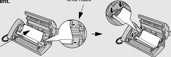
**7** Rotate the front gear as shown until the film is taut.
