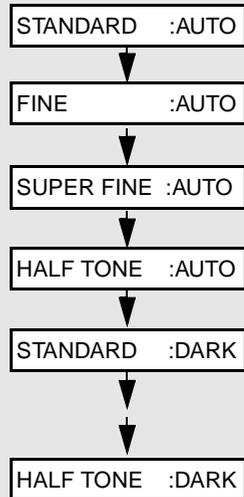
**Note:** In order to transmit in SUPER FINE resolution, the receiving fax machine must also have that resolution. If it doesn't, your machine will automatically step down to the next best available setting.
