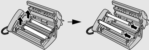
**3** Remove the two green gears from the spools. **DO NOT DISCARD THE TWO GREEN GEARS!**
