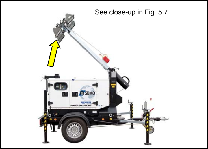
Figure 5.6 – Vertical positioning of column
