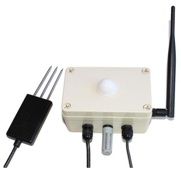
SZ3996B using the standard ZIGBEE Wireless Communication Interface, easy access to PLC, DCS and other instruments or systems for monitoring Illuminance, temperature, humidity, soil Moisture, soil
