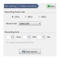
2 Set the [Recording frame rate], [Rec size], [Recording time], and the [Create compressed AVI file] option.
