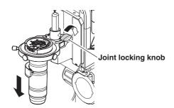
3 Align the O marks on the VH-Z20T and camera and rotate the camera clockwise until you hear a click.
