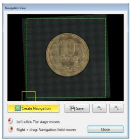
The green dashed line and the yellow solid line indicate the movable range of XY $\theta$  stage and the current position of XY $\theta$  stage, respectively.
