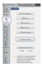
The [Vision correction] button turns yellow and the corrected image appears in the observation window.
