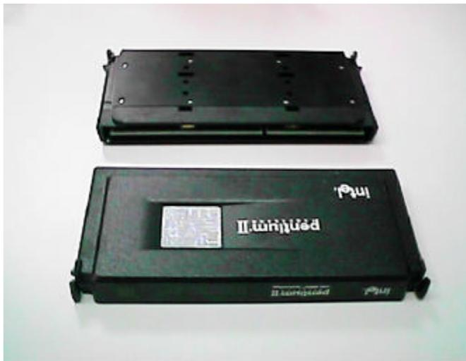
Figure 2:OEM Pentium® II Processor
