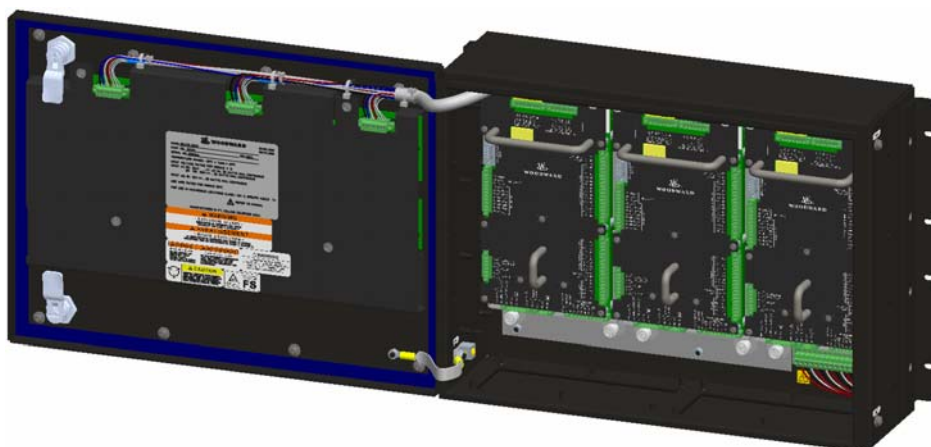
Figure 2-2. Typical ProTech-GII Bulkhead Package—Front Door Open
