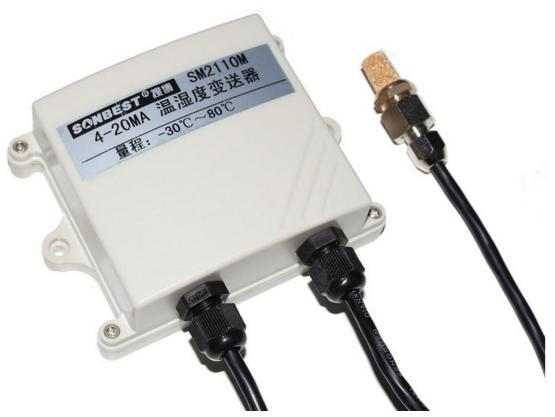
SM2110M-1 using the standard DC4-20mA current output signal, easy access to PLC, DCS and other instruments or systems for monitoring temperature, humidity state quantities. The internal use of high-precision sensing core and related devices to ensure high reliability and excellent long-term stability, can be customized RS232, RS485, CAN, 4-20mA, DC0~5V\10V, ZIGBEE, Lora, WIFI, GPRS and other output methods.
