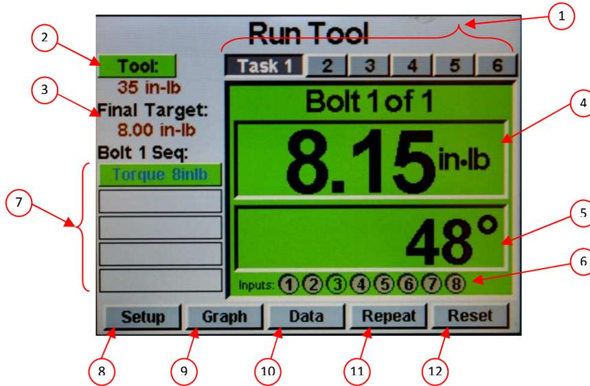
1. Quick Tap Task Keys: Allows the user to select one of 6 available tasks. Selecting these tabs will switch the tool to the selected task; settings for bolt counts, parameters, inputs, outputs, etc will switch with this action to the settings of that selected task.
