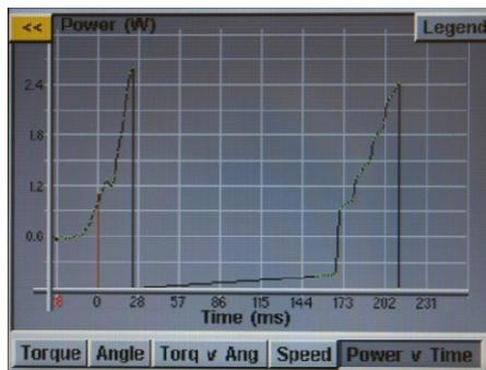
In each graph there is a 'Legend' button on the top of the screen. Tapping this button will affix labels to the lines overlaying each graph (where applicable) showing High Limits, Low Limits, Thresholds, etc as defined by the parameter of the rundown. The tool can be used while the controller displays the graph, just be aware that the graph will change with each cycle of the tool since the controller only stores the most recent rundown in graph form.
