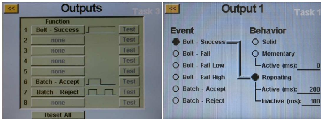
Select an available output button by tapping the 'none' button. Under the 'Event' heading, select the appropriate radio button. Select the type of output you would like under the 'Behavior' heading, and if necessary input the time intervals for the non-solid outputs. To adjust these values, tap on the number, enter the value you wish on the on-screen keypad, then tap the enter button. Any un-saved changes will appear in red until they are saved by exiting the screen with the yellow << button.
