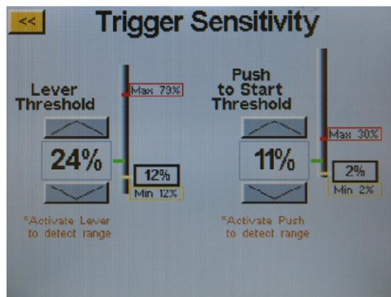
On the 'Trigger Sensitivity' screen there are two slider bars, one for the Lever, and one for the Push-to-Start. On each slider there is the following:
