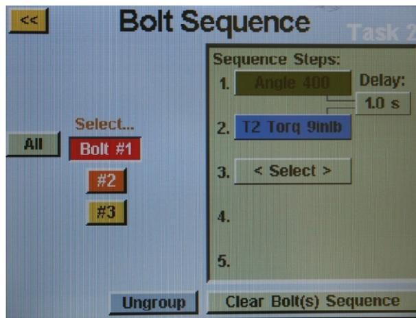
Each bolt can have up to 5 parameters assigned to run in sequence as well. A time delay between parameters may be programmed in this screen should the application require it. When the bolt count is 25 or less, each bolt can be selected separately to assign it any of the 8 available parameters on that task.
