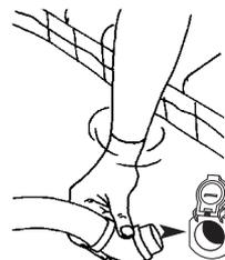
**Important:** To help prevent suction entrapment accidents, wall vacuum fittings should have a safety vac lock installed. Contact your builder or retail pool professional for details.
