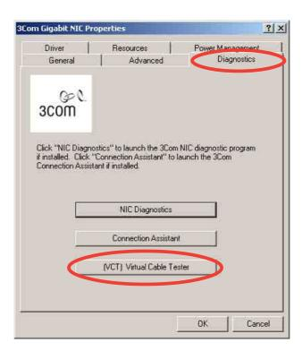
4. Click on the **(VCT) Virtual Cable Tester** button to display the following screen.
