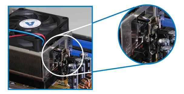
3. Align the other end of the retention bracket (near the retention bracket lock) to the retention module base. A clicking sound denotes that the retention bracket is in place.
