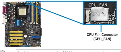
Don't forget to connect the CPU fan connector! Hardware monitoring errors may occur if you fail to plug this connector.
