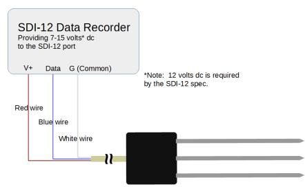
Diagram for a data recorder providing power to the SDI-12 port
