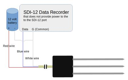
Diagram for the data recorder using an external battery
