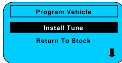
The pre-loaded tune option is the default menu option. Press the select key and you will be prompted to turn the key ON, which will start the tuning process.
