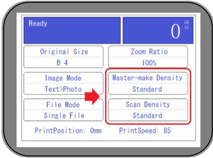
Generally, master making concentration and scanning concentration are set on [ Standard ] position, and will be also displayed in display screen. Different machine models will lead to different settings of printing pressure.
