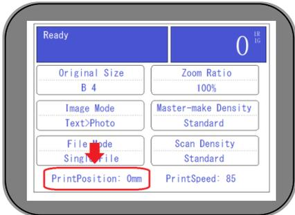
Adjust through [ Print position ] button of operation part. No matter the machine is stopped or working, adjustment is based on center. Moving scale displaced on the left lower portion of the display.
