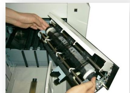
v ) Hold the paper core by one hand and dispose it to waste box.
