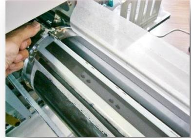
vi ) Disconnect the drum handle, and slightly rotate the drum to left.
