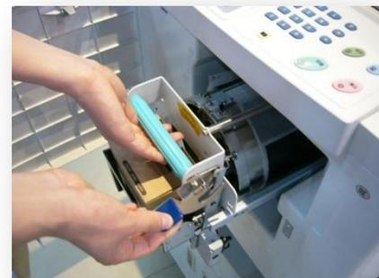
iv ) Hold the handle by one hand, and hold the drum frame by other hand and take out the drum.
