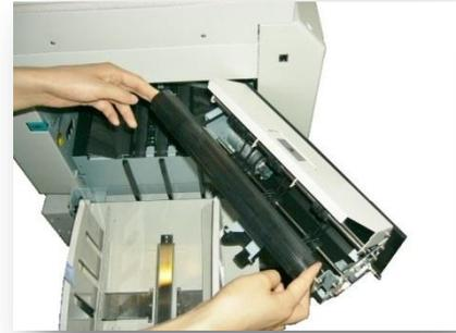
vii ) By pressing the upper cover, you will hear a sound of "bang" when it is locked.
