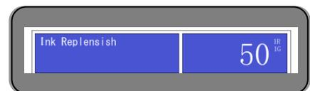
The machine will supply ink under proof printing state after master making. At this time paper feeding is terminated, and when drum is rotated, ink is supplied.
