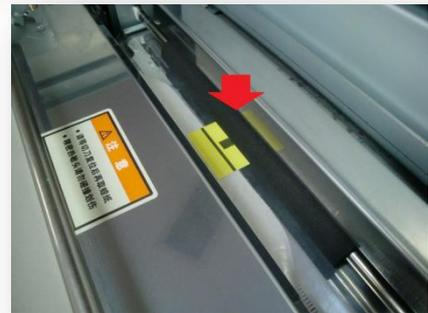
viii ) Pull the thermal head release lever to [ Close ] position.
