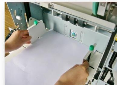
When printing position is adjusted to left ( Operation side )
