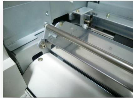
v ) Take down left and right master paper flanges on masterpaper core.
