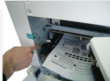
iii ) Press and hold [ Drum rotating button ] till [ Bang ] sound is made slightly. The drum will automatically stop when it reaches home position.
