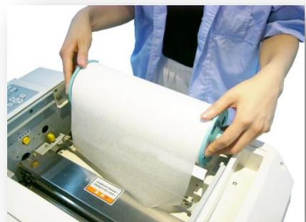
vii ) When master paper is put in master paper jack, continuously press cutter button.
