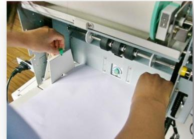
ii ) Moving left and right to adjust the right position of the papers
