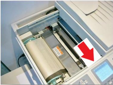
a : Thermal head release lever
