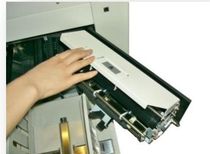
viii ) When the outer cover is closed, you will hear a sound of "cracking" when it is locked.
