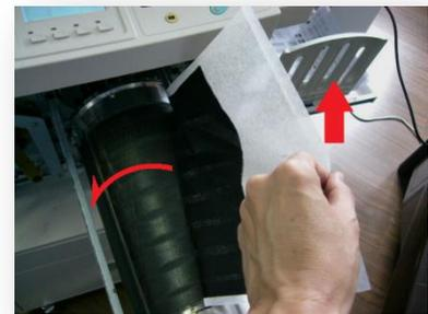
viii ) Rotate the drum to drum handle locking position.
