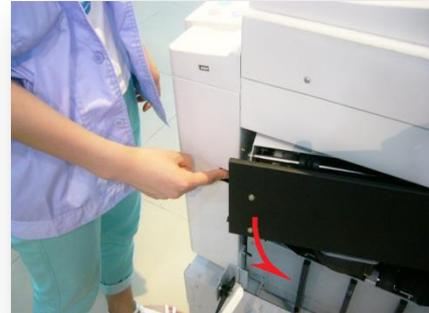
ii ) Press [ Drum rotating button ] to slowly rotate the drum and take out paper.
