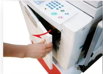
ii ) Pull drum mounting handle up, and unlock.
