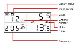
Single Channel measurement screen is shown.
