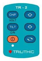
Toggles between Single Channel, Frequency mode, and Voltmeter function.
