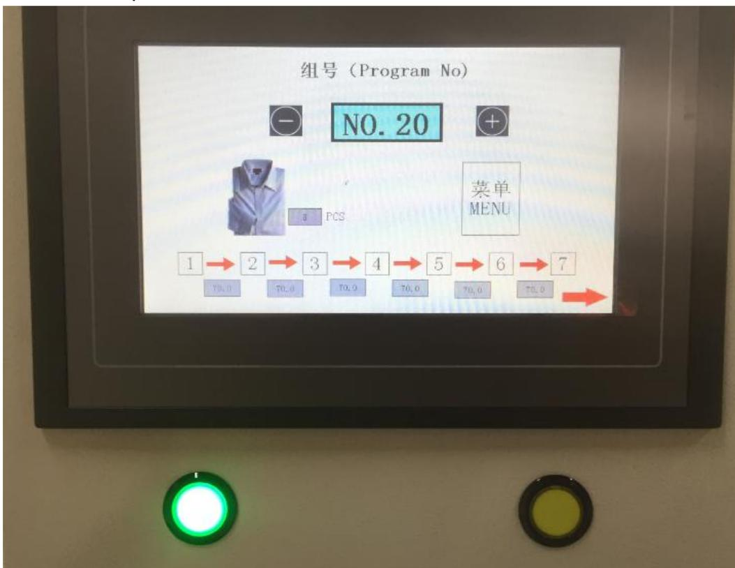
After power on, the green origin reset button at the bottom of the touch screen is in flashing state. After pressing, the reset operation of the origin reset button of the automation device is completed, and the button becomes normally on, as shown in the figure above.
