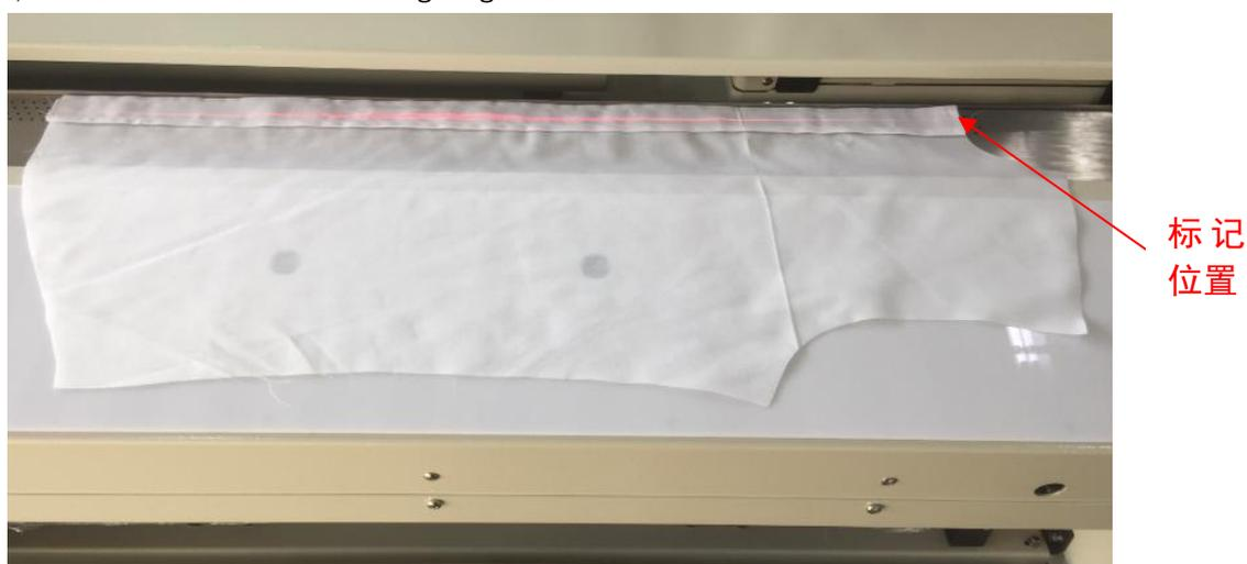
The neckline of the women's cloth piece is placed to the left, facing up, and the neckline is aligned with the mark of the mark position, as shown in the following
