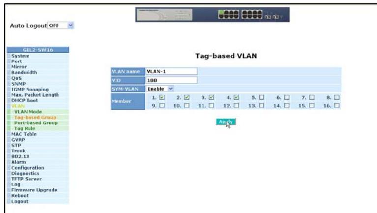
Figure 5.32 – Tag-based VLAN
