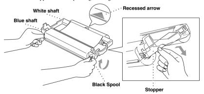
3 Turn the black spool on the right clockwise to tighten the ribbon.
