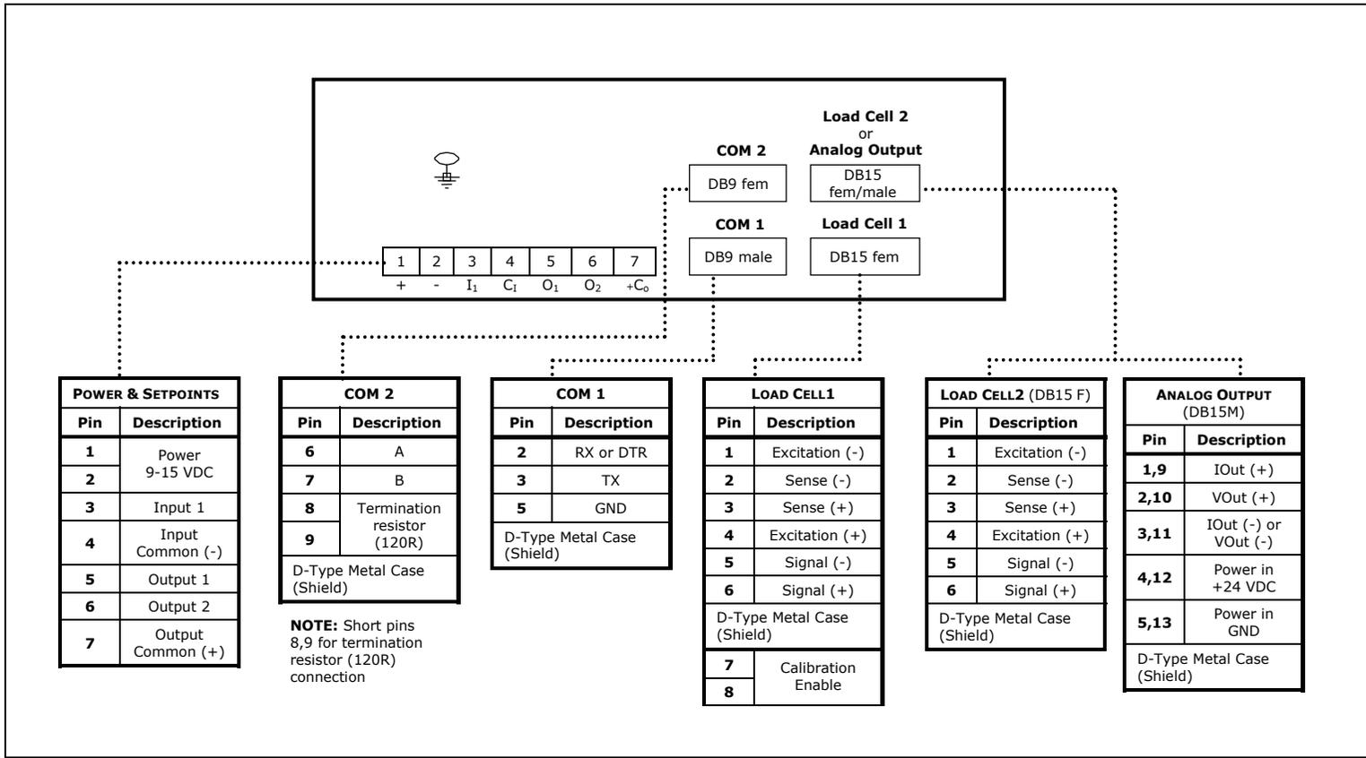
**iii. Terminal Connections (Wall-Mount Model)**
