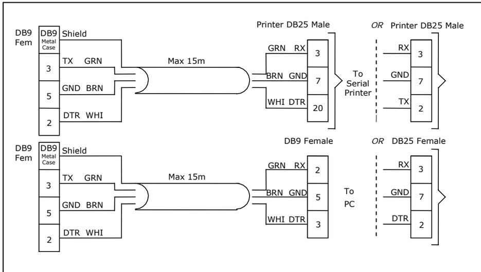
Figure 5 – Printer and PC cables connection diagram
