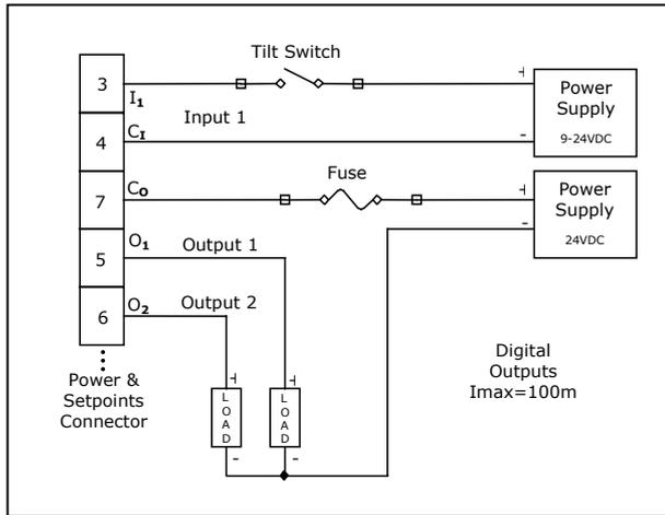
Figure 11 – Digital output and tilt switch connection diagram
