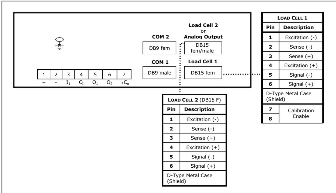
Figure 3 – Load cell connection diagram for desktop model
