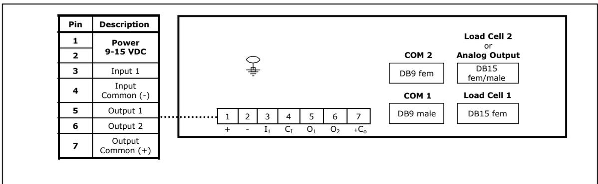
Figure 7 – Power cable connection diagram
