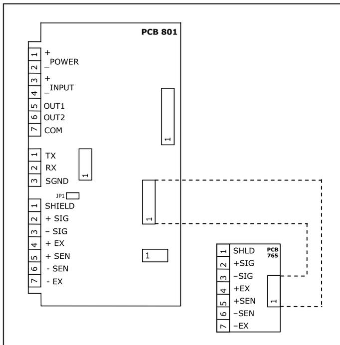
Figure 4 – Load cell connection diagram for wall-mount model
