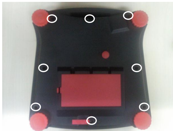
Figure 3-1. Screws (marked with white circles) that secure the housing.
