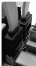
Connect the SATA data cables to both orange eSATAII connectors (eSATAII_BOTTOM (Port 5) and eSATAII_TOP (Port 4))
