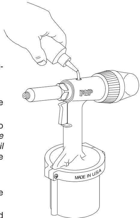
**Caution: Do not depress the trigger when Fill Screw 10 is loose. This will cause oil to be forced out under great pressure.**
