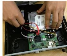
Connect the data wire and power wire as shown
