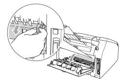
5 Pull the jammed paper out of the fuser unit. If the jammed paper cannot be pulled out easily, push down the blue tab with one hand as you gently pull out the paper with the other hand.
