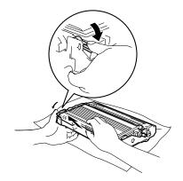
4 Put the toner cartridge back into the drum unit until you hear it lock into place. If you put it in properly, the lock lever will lift automatically.
