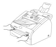
2 Using both hands put one sheet of paper in the manual feed slot until you feel the front edge of the paper touch the paper feed roller. Let go of the paper when you feel the machine feed the paper in a short distance.
