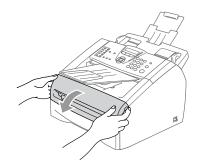
Pull out the drum unit and toner cartridge assembly.
