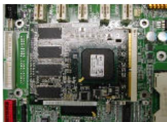
6. To remove the ZCR card just simply pull out the clips.
