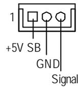
⚡ **Note** that when CPU FAN connector and Power FAN connector exist in the motherboard, you are **ONLY** allowed to connect either **CPU FAN 1** or **Power FAN**.
