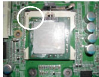
1. Pull the lever out, than lift up the Lever.
