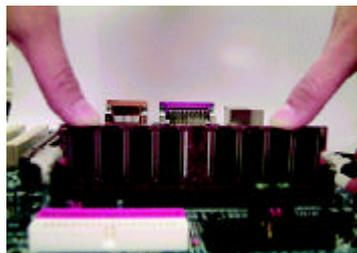
1. The DIMM slot has a notch, so the DIMM memory module can only fit in one direction.
