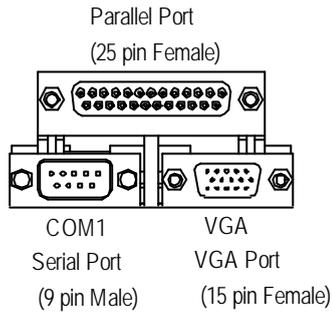
➤ This connector supports 1 standard COM port, 1 Parallel port and 1 VGA port. Device like printer can be connected to Parallel port; mouse and modem etc. can be connected to Serial ports.
