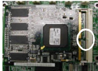
3. Insert the card into the connector by 60 degree and push it in until hearing 'click' sound.
