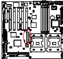
2. The ZCR connector has a notch, and the ZCR module can only fit in one direction.
