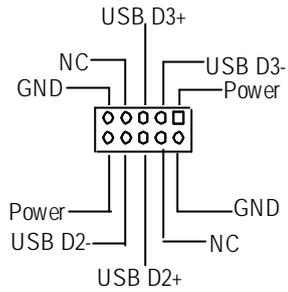
➤ Be careful with the polarity of the front panel USB connector. Check the pin assignment while you connect the front panel USB cable. Please contact your nearest dealer for optional front panel USB cable.
