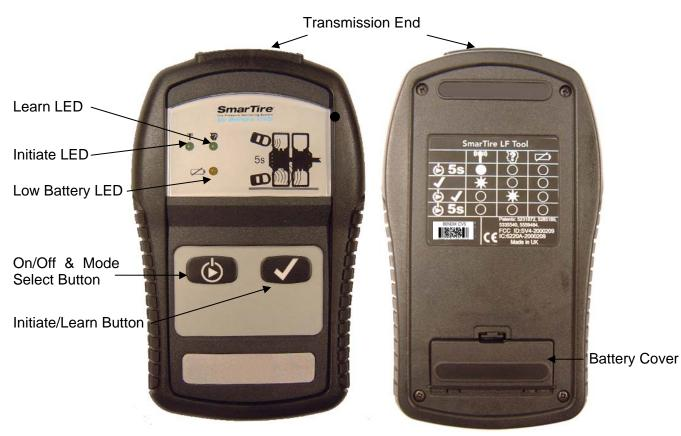
**Transmission End:** This part of the tool must be pointed towards the tire to initiate or learn a sensor.
