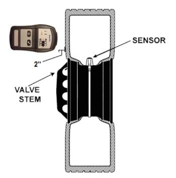
For dual-wheel assemblies, position the SmarTire<sup>™</sup> by Bendix CVS LF tool approximately 2 inches (5 cm) away from the tire's surface positioned at the center of the outboard tire's sidewall opposite the valve stem. The transmission from the tool will pass through the outboard tire and provoke a data transmission from the sensor mounted on the inboard tire.
