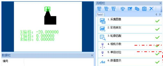
The screenshot shows the Kvision software interface. On the left, a window displays alignment data: X偏移: -20.000000, Y偏移: 0.000000, R偏移: 0.000000. On the right, a '流程栏' (Task List) window shows a sequence of tasks: 1. 采集图像 (Image Acquisition), 2. 彩色转灰 (Color to Grayscale), 3. 轮廓匹配 (Contour Matching), 4. 相机示教 (Camera Teaching), 5. 单目对位 (Single-camera Alignment), and 6. 数值显示 (Numerical Display). Red dashed arrows point from the '相机示教' and '单目对位' tasks to explanatory text on the right.
