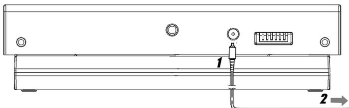
**1** Connect the output plug of AC/DC adapter to the battery pack.
