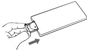
**2** Remove the old battery, then insert the new battery into the battery holder with the + side facing upwards.
