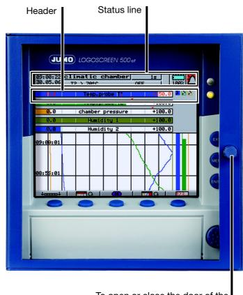
To open or close the door of the instrument, turn the knob
