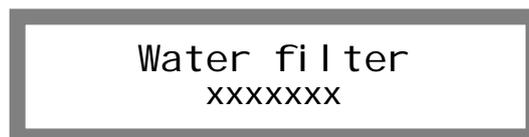
The display will show the option "WATER FILTER". You have to select the number of liters of water for the "WATER-SOFTENER" regeneration/replacement alarm. When the number of liters selected arrive to the number of this option, the alarm advice of the water filter regeneration/replacement.
