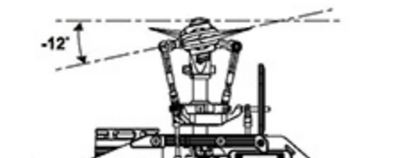
Stick Position at Low/Throttle 100%/Pitch -12° 搖桿低油門100%/Pitch-12°
