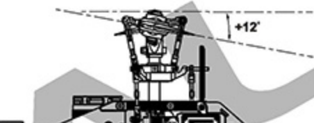
Stick Position at High/Throttle 100%/Pitch +12° 搖桿高油門100%/Pitch+12
