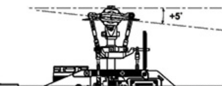
Stick Position at Hovering/Throttle 70%/Pitch +5° 搖桿停懸/油門70%/Pitch+5
