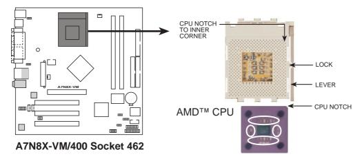
Each AMD CPU has a "marked" corner. This corner is usually indicated with a notch, and/or a golden square or triangle. Refer to this indicator while orienting the CPU. A fan and heatsink should be attached to the CPU to prevent overheating.
