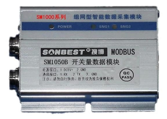
SM1050B using the standard RS485 bus MODBUS-RTU protocol,easy access to PLC,DCS and other instruments or systems for monitoring 开关量 state quantities. The internal use of high-precision sensing core and related devices to ensure high reliability and excellent long-term stability, can be customized RS232,RS485,CAN,4-20mA,DC0~5V\10V,ZIGBEE,Lora,WIFI,GPRS and other output methods.
