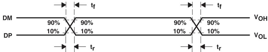
NOTE: The  $t_r/t_f$  ratio is measured as  $t_r(DP)/t_f(DM)$  and  $t_r(DM)/t_f(DP)$  at each crossover point.
