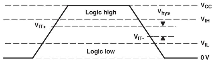
Figure 4. Single-Ended Receiver Input Signal Parameter Definitions
