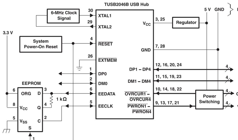
Figure 9. Typical Application of the TUSB2046B USB Hub
