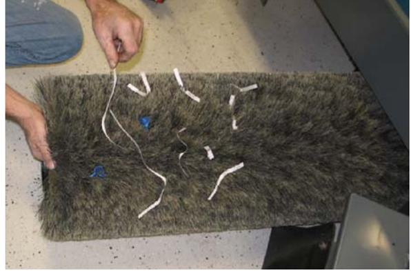
Check the main brush pattern and rotate the brush end-for-end after every 50 hours of operation, for maximum brush life and best sweeping performance. Refer to *REPLACING OR ROTATING THE MAIN BRUSH*.
