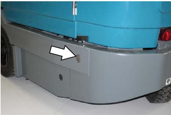
9. Route the tie-downs to the opposite ends of the machine and hook them to the brackets on the floor of the trailer or truck. Tighten the tie-down straps.
