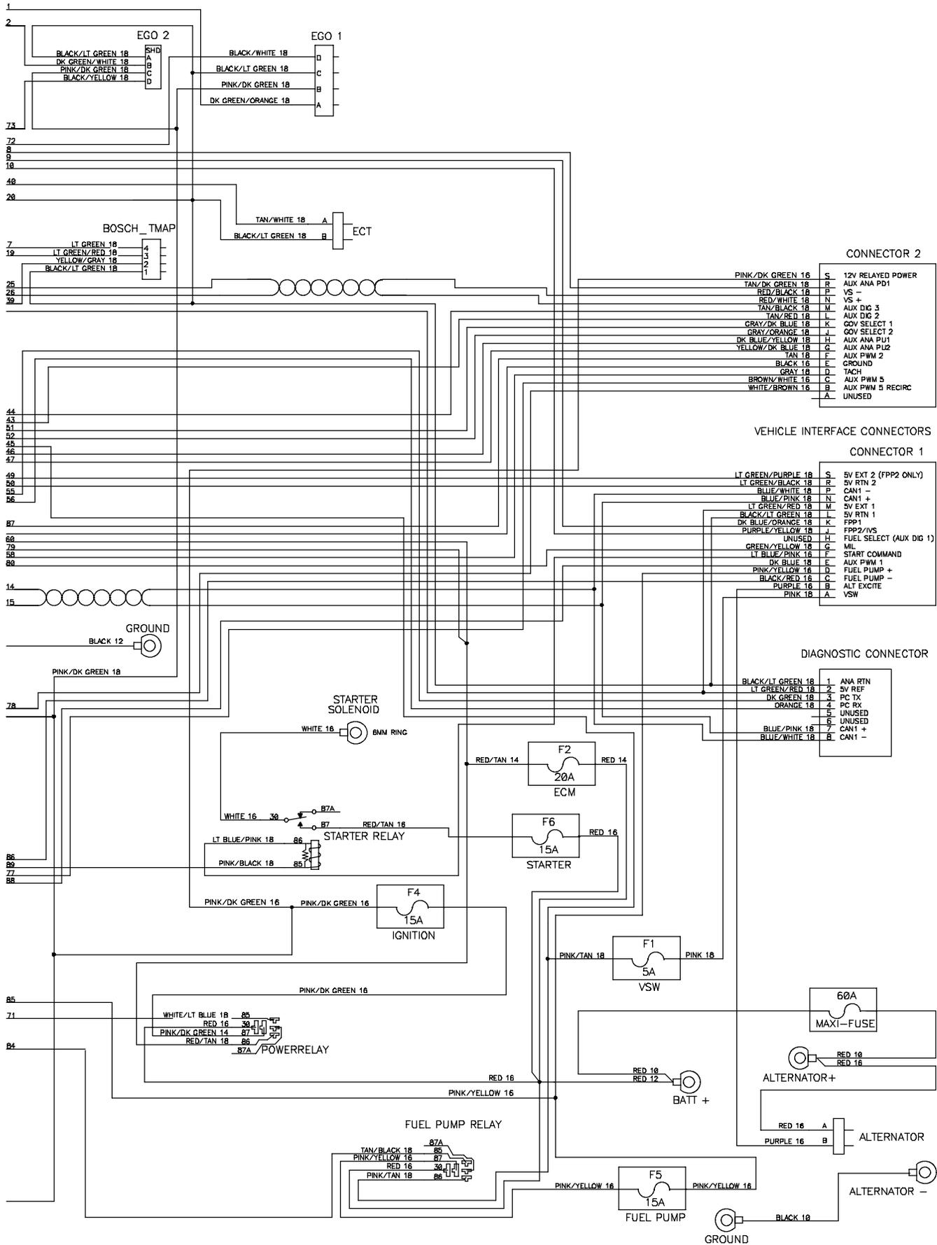
LPG Engine Harness Electrical Schematic (1 of 2)
