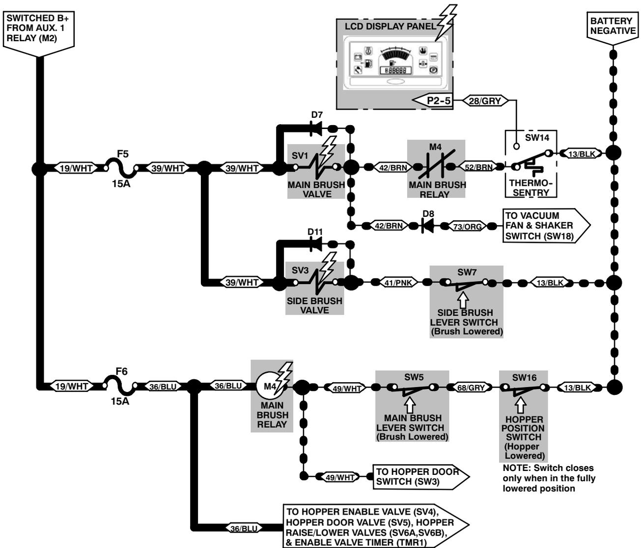
**i** Thermo-Sentry switch (SW14) is shown in the normal NON-activated position (13/BLK connected to 52/BRN). The switch is activated (13/BLK connected to 28/GRY) when the Hopper air temperature exceeds 71°C (160°F). The Hopper Fire indicator on the LCD panel will also illuminate when this switch is activated. When the temperature falls below 60°C (140°F), the switch will return to the NON-activated position, and the indicator light will turn OFF.
