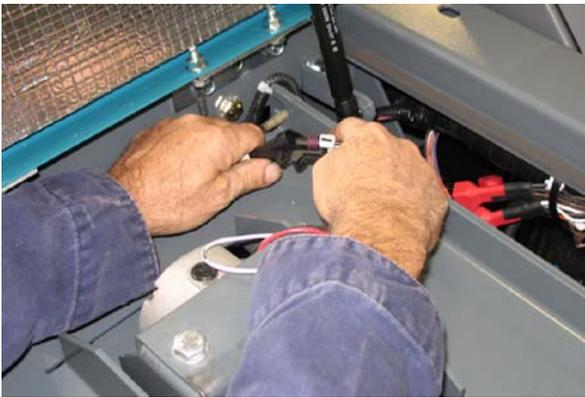
3. Remove the filter shaker assembly from the filter housing.
