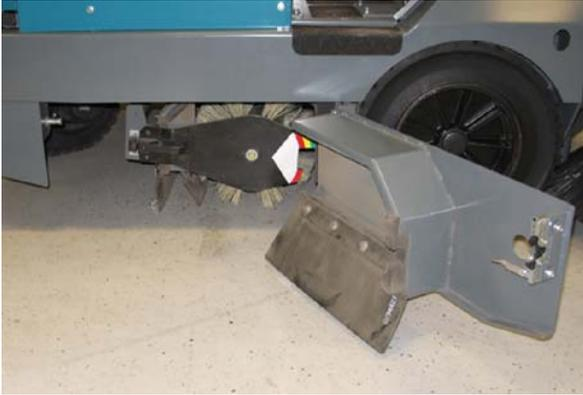
3. Unlatch and remove the brush idler plate.
