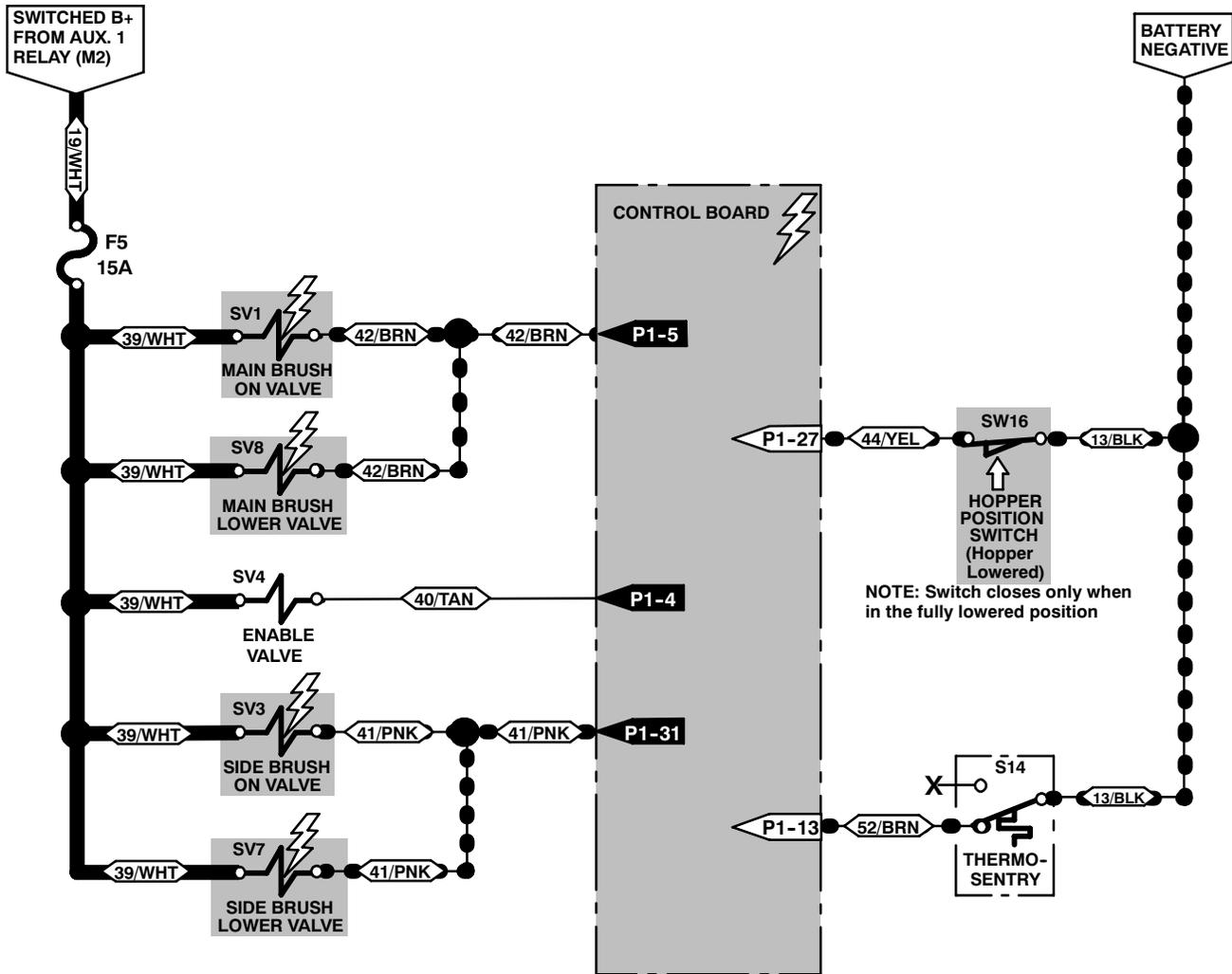
**i** Thermo-Sentry switch (S14) is shown in the normal NON-activated position (13/BLK connected to 52/BRN). The switch is activated (13/BLK connected to 28/GRY) when the Hopper air temperature exceeds 71°C (160°F). The Hopper Fire indicator on the control panel will also illuminate when this switch is activated. When the temperature falls below 60°C (140°F), the switch will return to the NON-activated position, and the indicator light will turn OFF.
