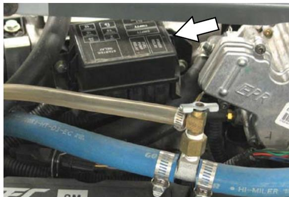
**NOTE:** Always replace a fuse with a fuse of the same amperage.
