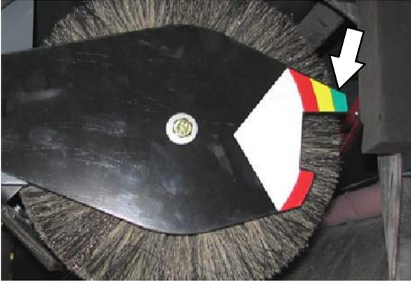
2. Loosen the main brush adjustment knob and slide the pointer so it matches the color band on the brush idler plate. Retighten the knob.
