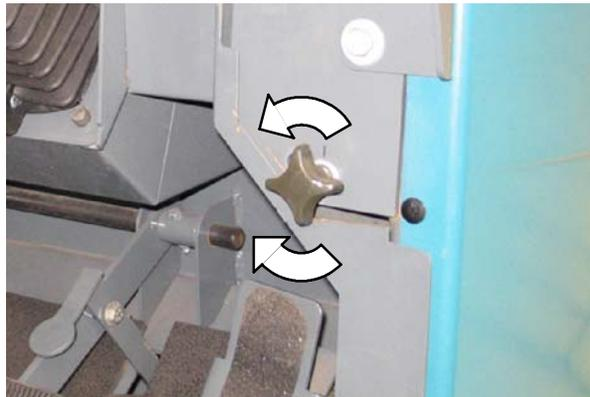
**S30XP and S30X4:** Tighten the *side brush adjustment knob* into the side brush bracket to increase the brush pattern and loosen the knob to decrease the brush pattern.
