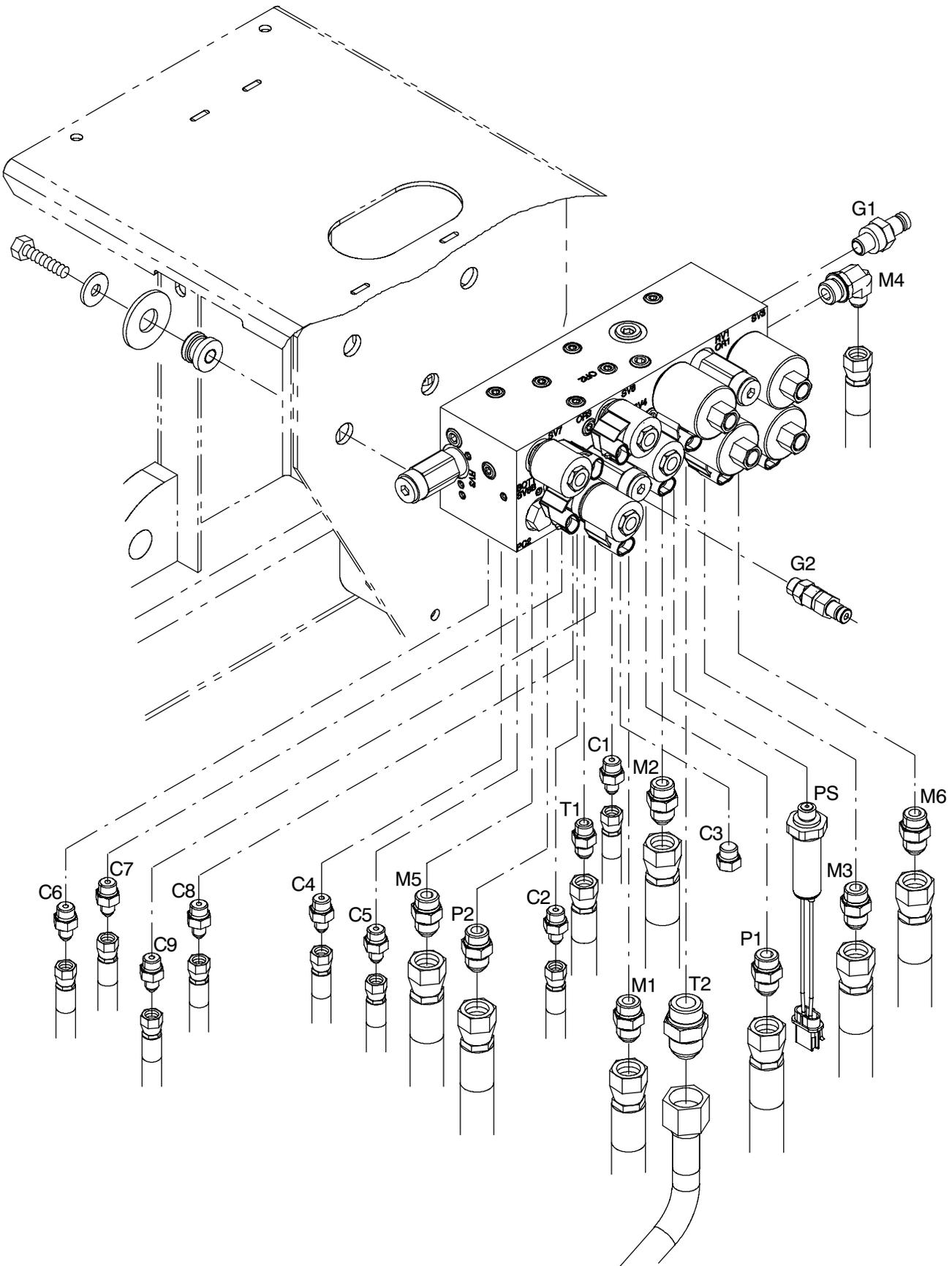
Hydraulic Priority and Flow Divider Valve Diagram (S30X4)
