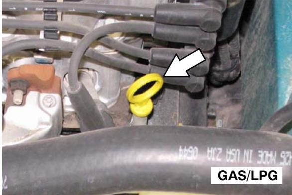
Gas/LPG engines: Fill the engine with oil until the oil is between the indicator marks on the dipstick. DO NOT fill past the top indicator mark. The engine oil capacity is 3.5 L (3.7 qt) with oil filter.
