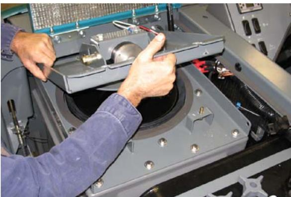
4. Remove the dust filter from the filter housing.
