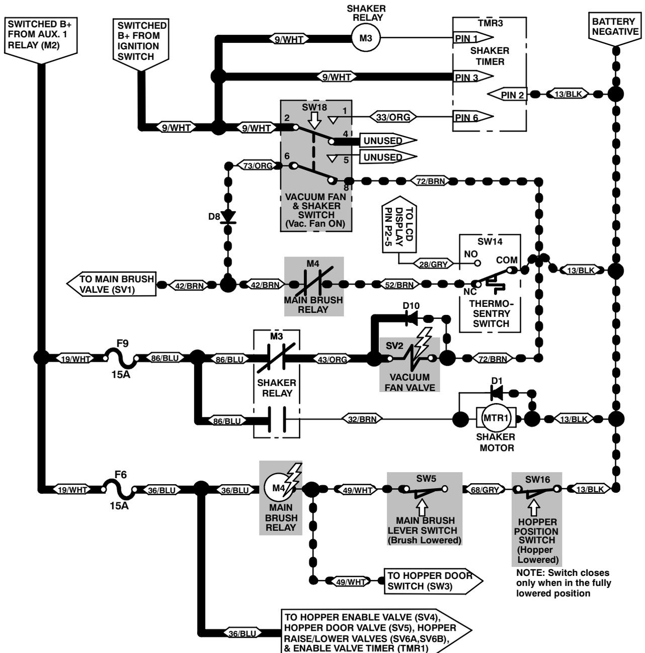
**i** - The Thermo-Sentry switch (SW14) is shown in the normal NON-activated position (13/BLK connected to 52/BRN). The switch is activated (13/BLK connected to 28/GRY) when the Hopper air temperature exceeds 71°C (160°F). The Hopper Fire indicator on the LCD panel will also illuminate when this switch is activated. When the temperature falls below 60°C (140°F), the switch will return to the NON-activated position, and the indicator light will turn OFF.
