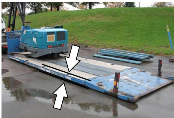
4. To winch the machine onto the truck or trailer, attach the winching chains to the holes in the right and left lower corners in front of the machine.
