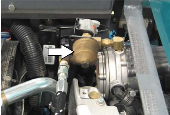
Disassemble the fuel lock off valve to access the LPG fuel filter.
