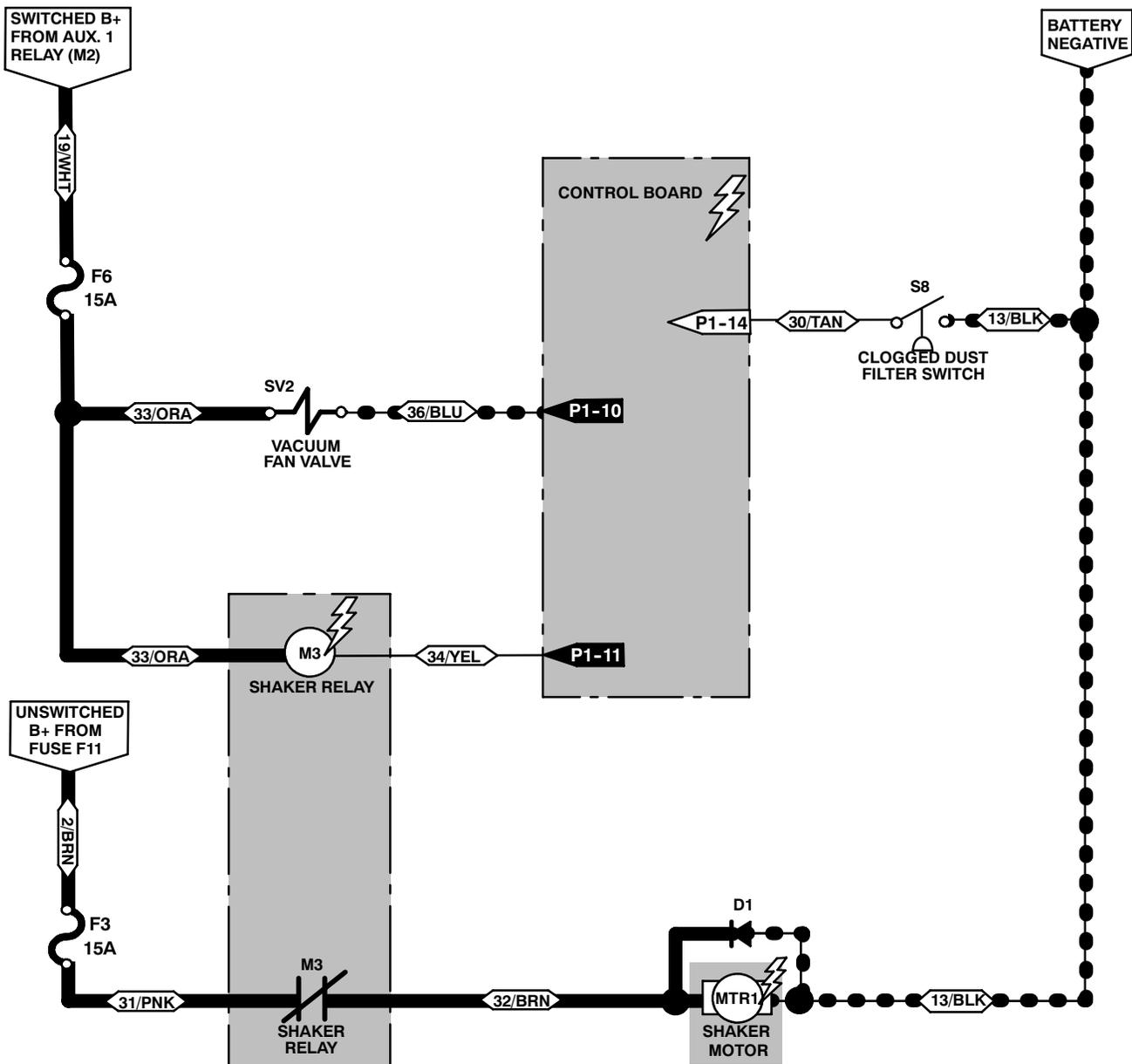
**i** - When activated, the Shaker System will run for 30 seconds. The Shaker System is automatically activated when turning the sweeping system OFF, or can be activated anytime by pressing the Shaker button. Pressing the Shaker button during sweeping will turn OFF the Vacuum Fan during the Shaker cycle. The Shaker System is the only sweeping related function that can be activated with the Hopper in the raised position.
