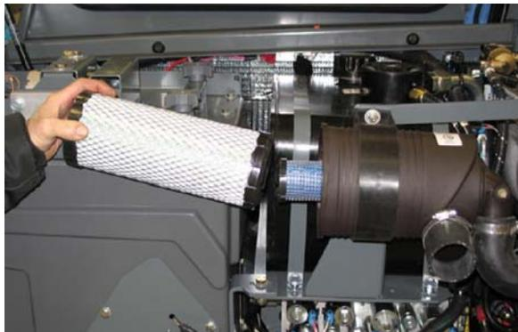
Replace the safety filter element after the primary has been changed three times. Do not remove the safety filter element from the housing unless it is restricting air flow.
