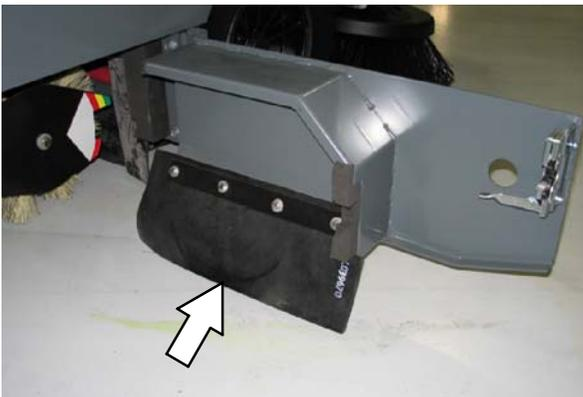
*NOTE: The brush door skirts have slotted holes to allow for a ground clearance adjustment. The door must be closed for proper adjustment.*
