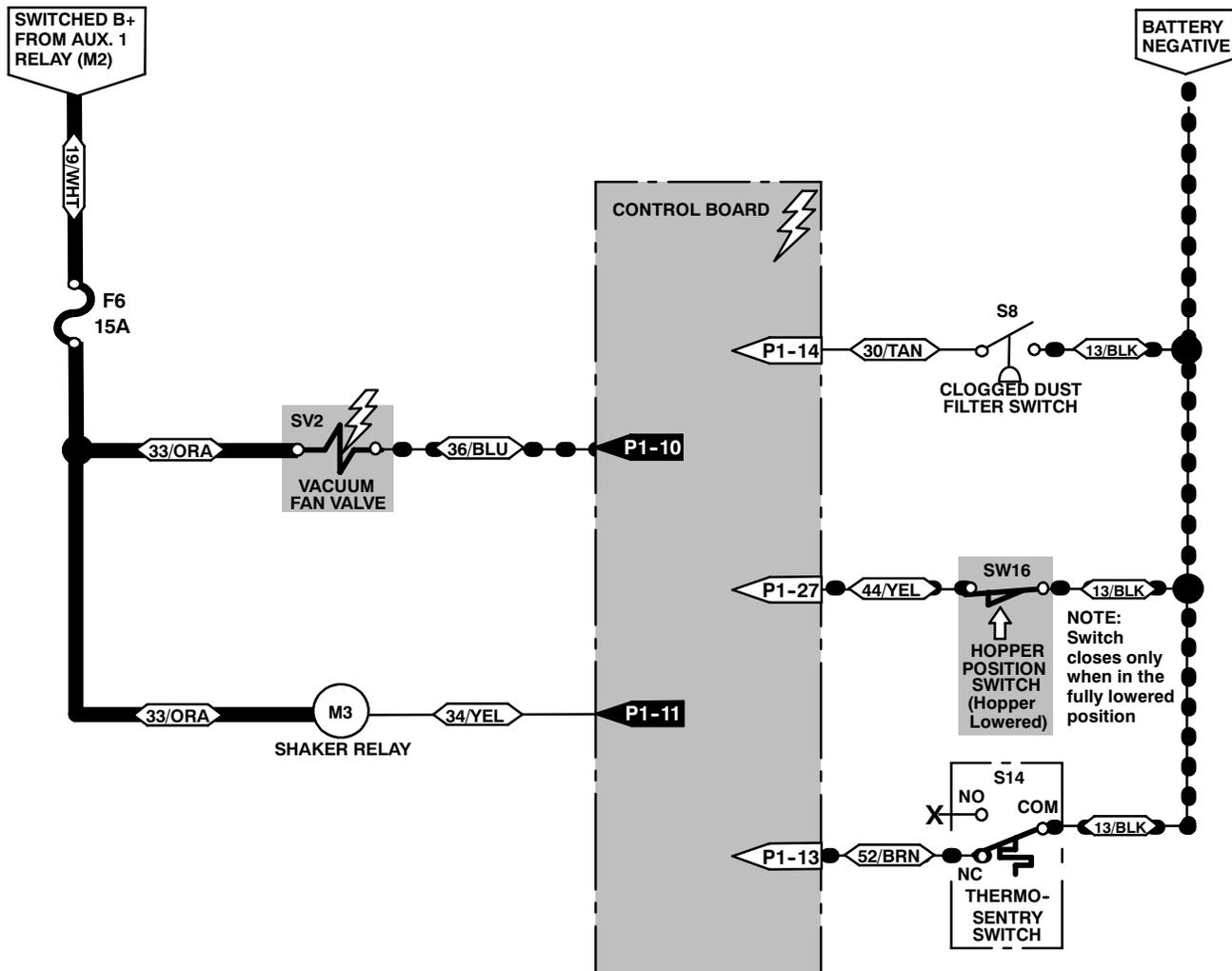
**i** - Thermo-Sentry switch (S14) is shown in the normal NON-activated position (13/BLK connected to 52/BRN). The switch is activated (13/BLK NOT connected to 52/BRN) when the Hopper air temperature exceeds 71°C (160°F). The LCD screen on the control panel will also show “F5: HOPPER FIRE” when this switch is activated, all sweeping functions will turn OFF and the hopper door will close. When the temperature falls below 60°C (140°F), the switch will return to the NON-activated position.
