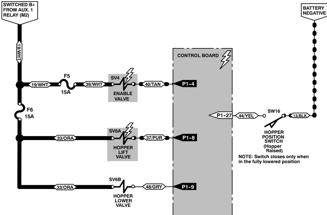
**i** - The Enable Valve (SV4) is ON ONLY during the following Hopper related functions:
