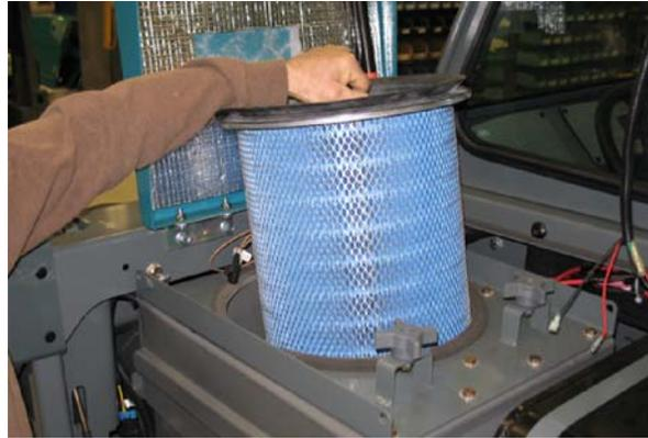
5. Clean or discard the dust filter element. Refer to *CLEANING THE DUST FILTER*.
