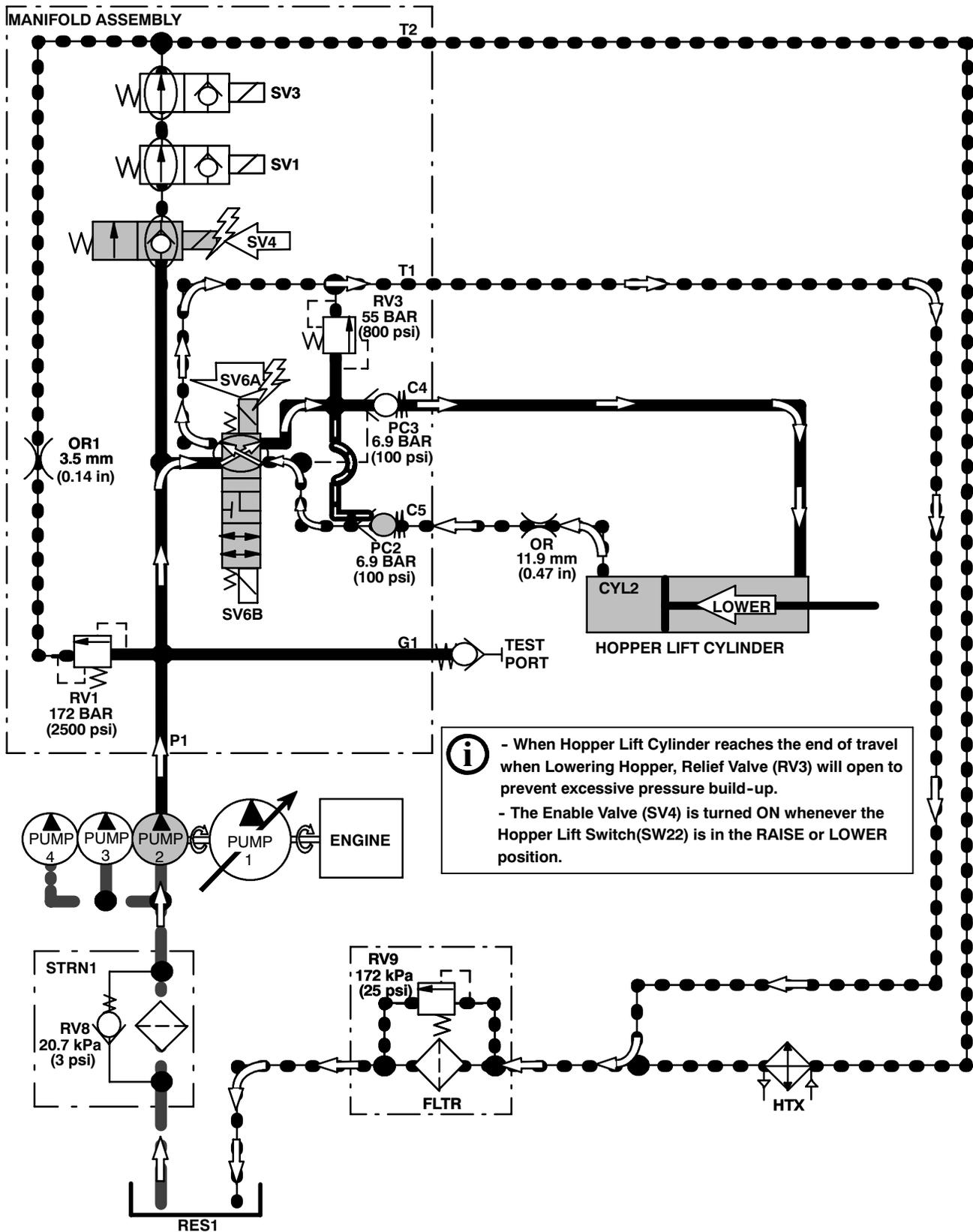
**i** - When Hopper Lift Cylinder reaches the end of travel when Lowering Hopper, Relief Valve (RV3) will open to prevent excessive pressure build-up.
