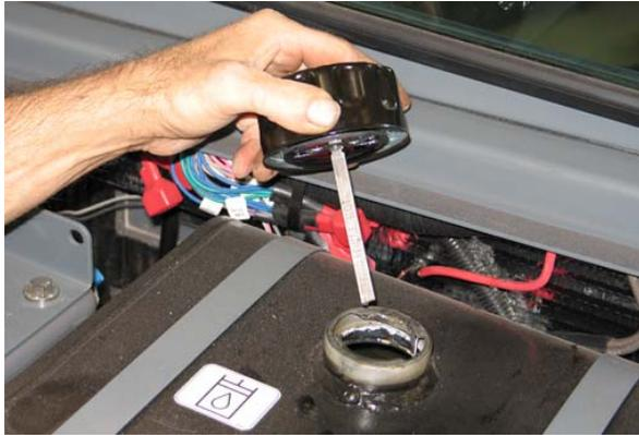
A filler cap is mounted on top of the reservoir. It has a built-in breather and fluid level dipstick. Replace the cap after every 800 hours of operation.
