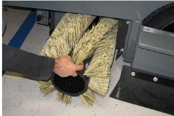
5. Replace or rotate the main brush end-for-end.
