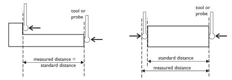
For Example: To check the scale against a standard which is exactly 500mm wide:
